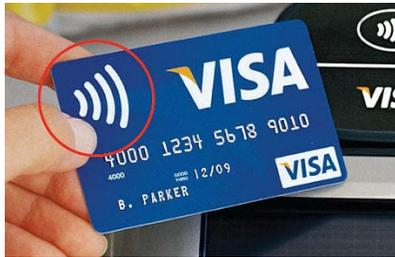
Some debit and credit cards have an RFID chip inside of them (though most do not) and are usually identified by a symbol printed on the card, such as the one pictured here.
